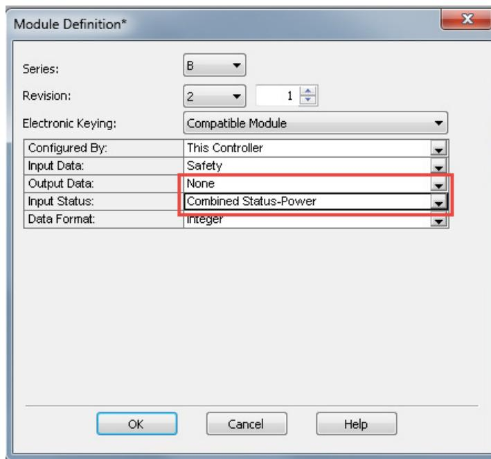
Setting the output data to None means that you cannot use the Test Outputs as standard output, which is appropriate in this example. This arrangement saves one controller connection because we are using only the input connection.
