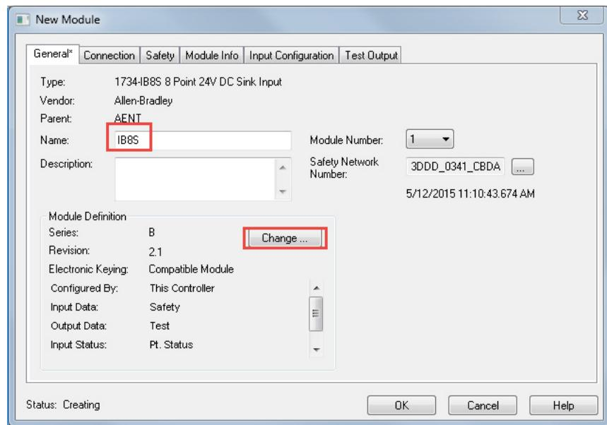
13. When the Module Definition dialog box opens, change the Output Data to None, verify that the Input Status is Combined Status-Power, and click OK.
