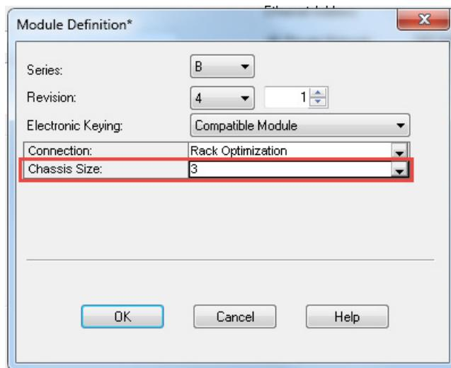
Chassis size is the number of modules that are inserted in the chassis. The 1734-AENT adapter is considered to be in slot 0, so for one input and one output module, the chassis size is 3.
