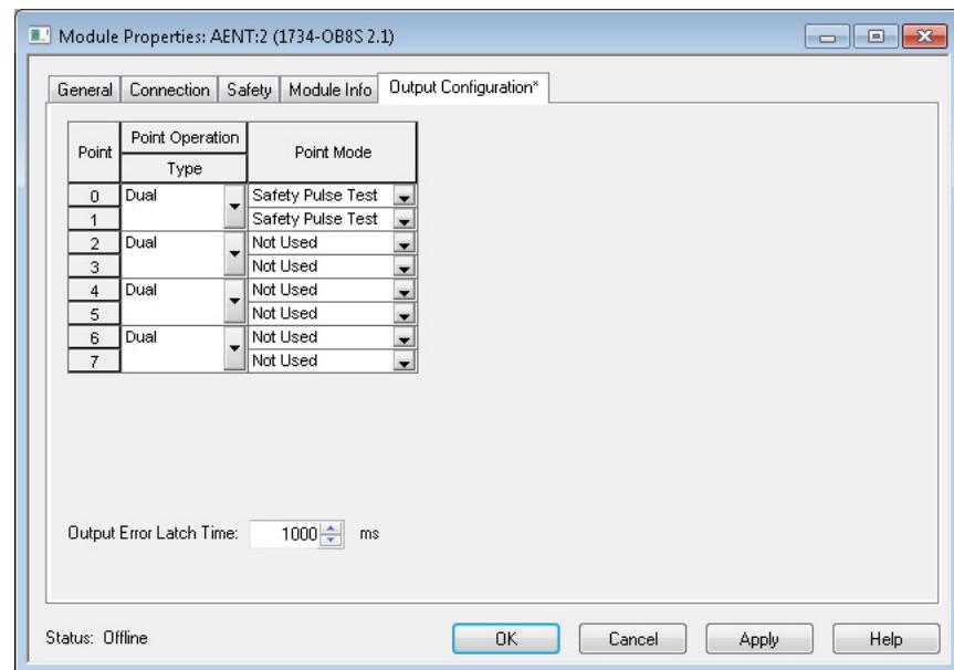
The electromechanical coil on the contactor (outputs 0 and 1) can be pulse tested without reacting to the brief low (0) pulse. If you are using a contactor that does react to the pulse test, then it is advisable to disable the pulse test. This arrangement should not degrade the overall safety rating of redundancy and monitoring that are being used.
