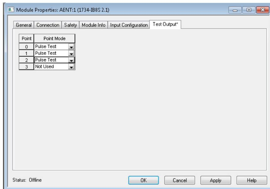
T0 and T1 are being used to pulse test both the Trojan 5 door interlock switch and the enabling switch channels. T2 is being used to pulse test the contactor feedback circuit.
