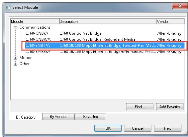
4. Name the Module module, type its IP address, and click OK.
