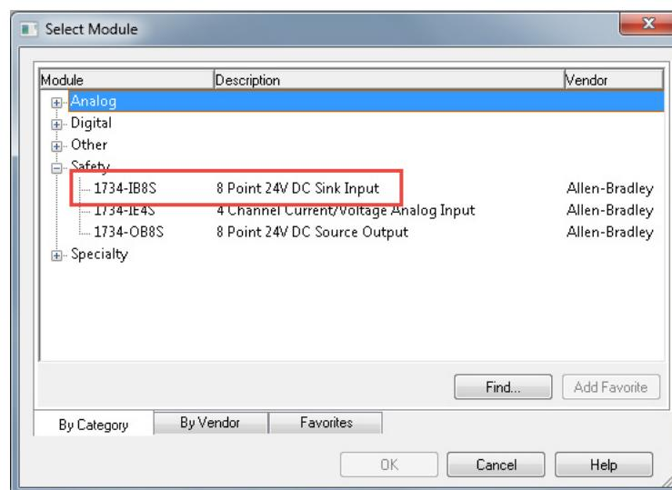
12. In the New Module dialog box, name the device IB8S, and click Change.
